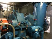
Motor Top Gas Compressor 2500 kw 3000 RPM Unit 40 Gearbox and Compressor 10434 RPM
