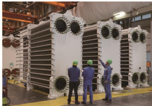
LX-160, one of the largest plate heat exchangers in the world
