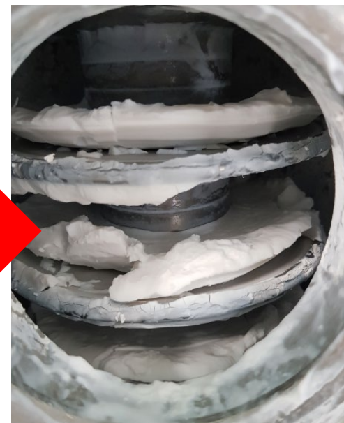
Before discharge (Solid content = 35wt%)
