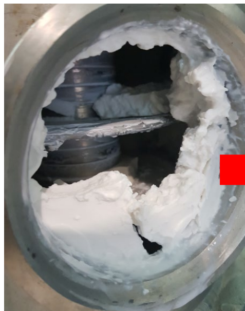
After discharge -> sticky (Solid content = 25wt%)
