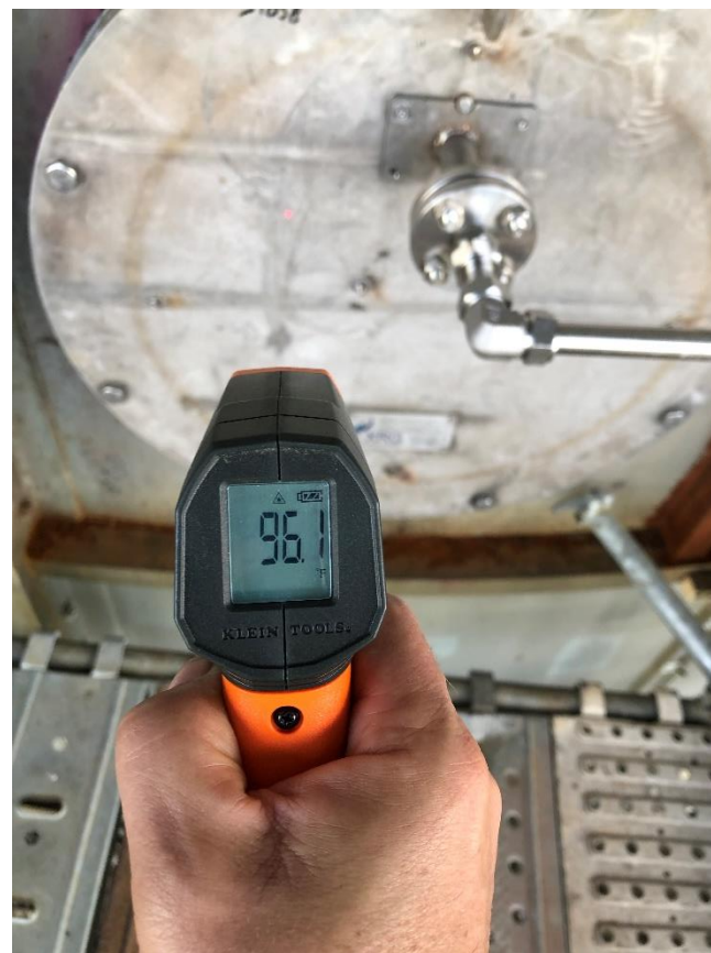
Xceed front plate temperature (96°F = 35°C)
