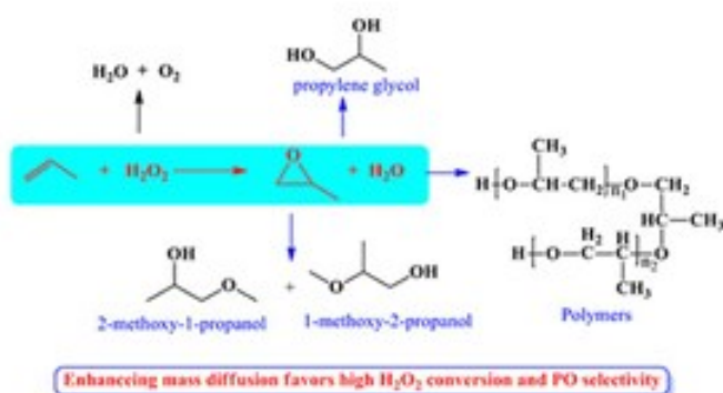
FIG. 4. The main epoxidation reaction and side reactions, including \text{H}_2\text{O}_2 decomposition, ring-opening and polymerization of PO product in the HPPO process.
