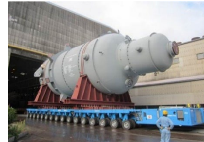
Large-scale reactor (Shell & Tube) maximum capacity: 275kt/y (EO)
