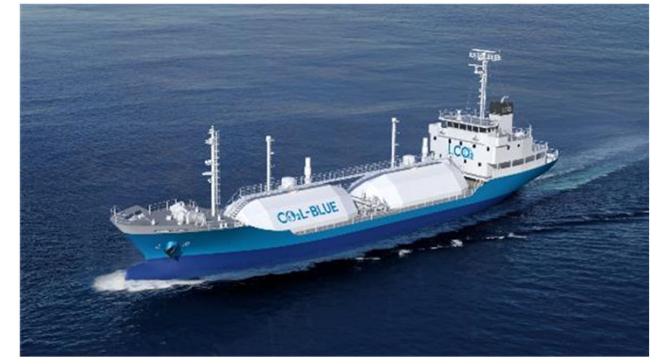
Liquefied CO 2 carrier demonstration test ship
