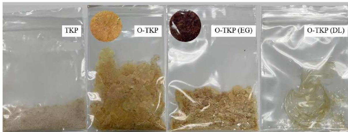
Fig. 2 Images of the samples after drying at 60° C and storing for 30 days (small circle images).
