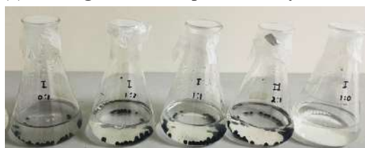
(a) During batch adsorption in dialysate solution
