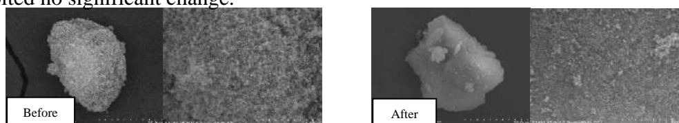
Fig. 1 The SEM image of Cab-Si and Cab-Si after impregnation with 1% Ga, respectively
