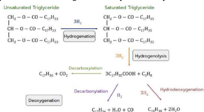
Fig. 1 Reaction of green diesel production from triglyceride and fatty acid [4]
