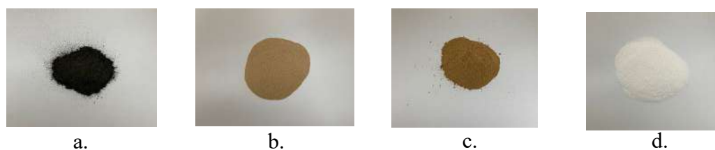
Fig. 1. Physical appearances of a. raw SCBA, b. SCBA-derived leached ash, c. SCBA-derived extracted ash and d. SCBA-derived mesoporous silica (SCBA MPS).
