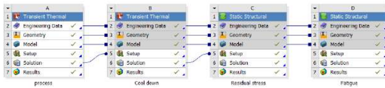
Fig. 3 ANSYS Work Bench schematic for solving for thermo-mechanical fatigue.
