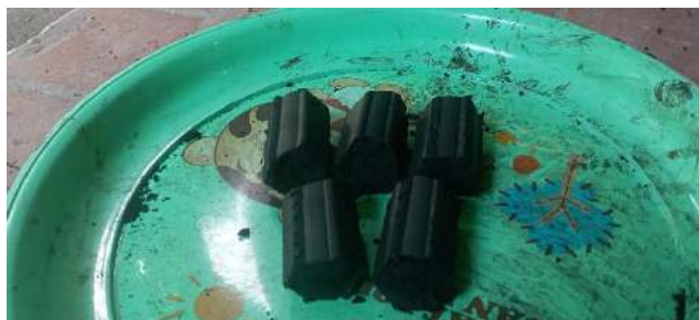
Fig. 3 Solid fuel from the charcoal compressor.
