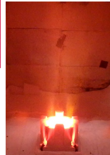
COOLstar BURNER FIRING 100% H 2
