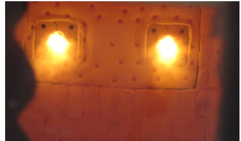
Down fired DFR (staged-air) burners firing 100% NH 3 as our test facility in Luxembourg.
