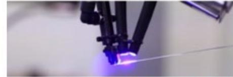
Continuously wound carbon fiber in epoxy matrix through additive process
