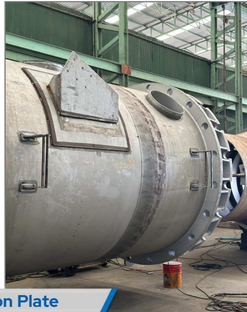
Shell nozzle fit-up / welding
