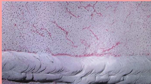
4 Pitting & Cracking (SCC with branch)
