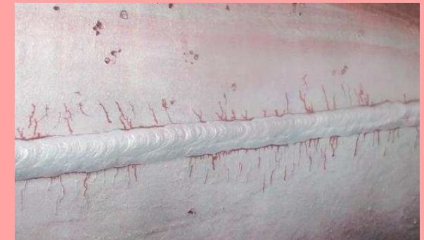
4 Pitting & Cracking (SCC with branch)
