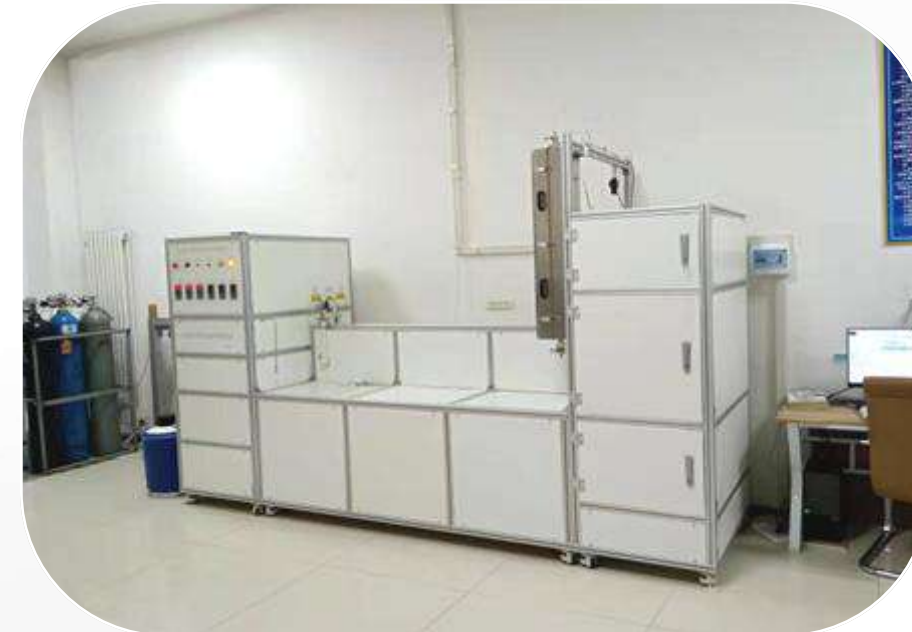
Evaluation device of Diesel vehicle exhaust denitrification catalyst
