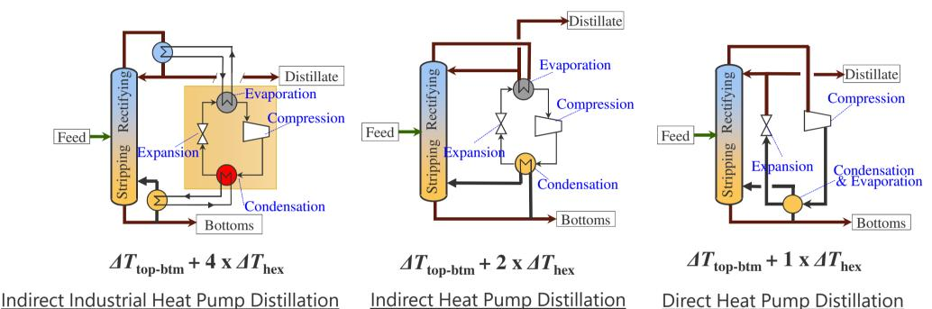
• Acceptable temperature rise in heat pump system = "Less than 30 deg C" •  $\Delta T_{hex}$ : 5~10 deg C  $\rightarrow$  2 x  $\Delta T_{hex}$ : 10~20 deg C, 4 x  $\Delta T_{hex}$ : 20~40 deg C
