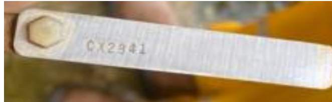
Mild Steel Coupon – Pass Copper Sulphate test
